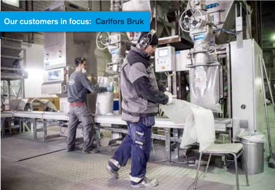
Stefan Nolic and Allan Bakr working with one of the bag filler at Carlfors Bruk, Sweden. Currently, the company has two Manpac bag fillers from Vebe Teknik, which can be quickly swapped round to pack various types of content.
